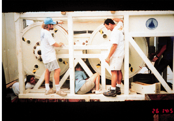
Figure 8: Threading Wire Through Winch
