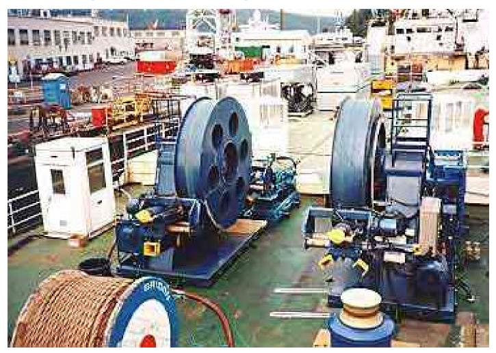
CONTROLLED PICKUP: 133440N (30000 lbf) @ 1.7 KTS CONTROLLED PAYOUT: 89250N (20000 lbf) @ 3 KTS
