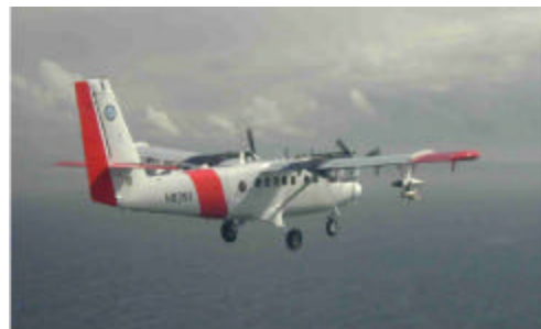
Figure 1. The CIRPAS UV-18A “Twin Otter” turboprop research aircraft. This twin turboprop Short Takeoff and Landing (STOL) aircraft can cruise at low speeds for long durations over the ocean with a maximum endurance of 8 hrs, maximum
