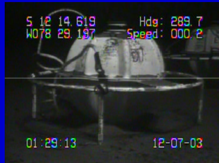
Precision transponder viewed from seafloor survey package.
