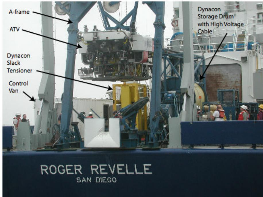
ATV was transferred from Navy to SIO in 2000. It is a heavy duty work vehicle (200+ lbs payload) capable of working to 6100 m depth. As shown in the photograph it has a pair of manipulators, video cameras, lights and sonar systems.
