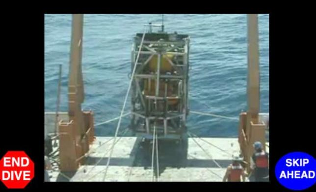
OK. Here we go! The ROPOS underwater vehicle begins each dive inside a garage. The garage is lifted off the deck of the ship and lowered into the water on a long fiber optic cable. It usually takes ROPOS about 2 hours to descend to the top of Axial Seamount, which is almost a mile below the surface, but we'll speed it up a bit here.
