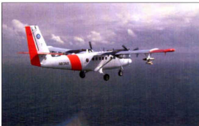
Fig. 1. The CIRPAS UV-18A Twin Otter turboprop research aircraft. This twin turboprop Short Take-off and Landing (STOL) aircraft can cruise at low speeds for long durations over the ocean with a maximum endurance of 8 hours, maximum altitude of 7600 m, 35–80 m/s operational speed range, 200 amps of payload power and an approximately 2400 kg useful load.
