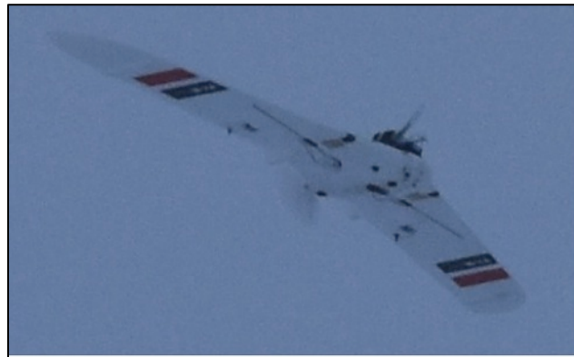
Fixed wing UAS with radiosonde on top.
