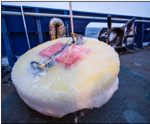
WaveBuoy 02: an example of the heavy icing during the deployment
