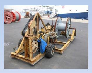
Note: most of this equipment is 1960's vintage; no capability for precise level winding or tensioning.
