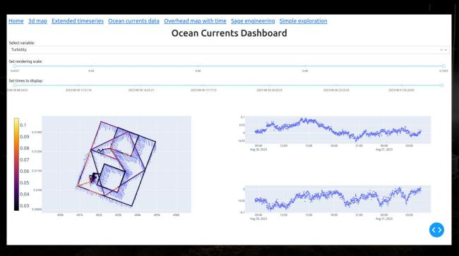
Transmitted data is aligned with spatial location by interpolating queue messages with USBL pings.
