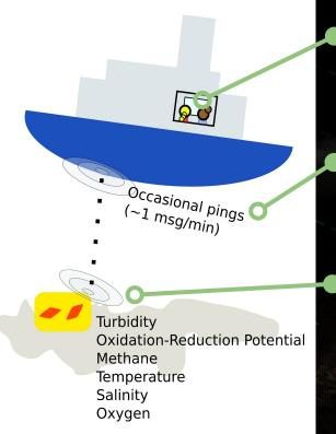
Local network on the ship established for AUV Sentry operations; network broadcasts vehicle data and repeats ship-side USBL navigation messages.
