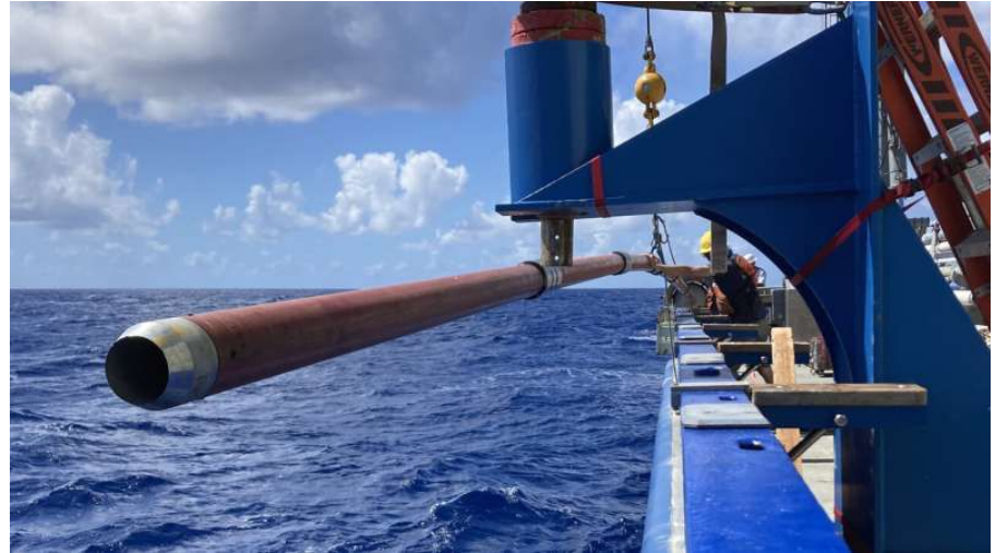
Sediment long corer deployed from the R/V Neil Armstrong in the Puerto Rico Trench to a depth of 8,385 meters
