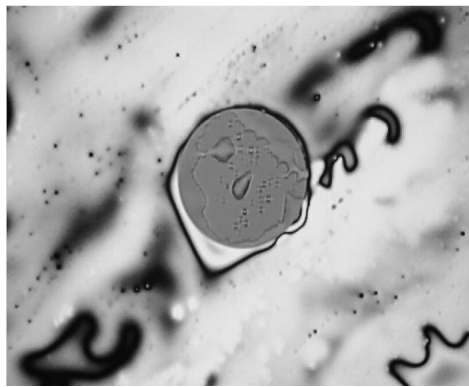
Launch fiber endface 1: quick clean pen, 2 pushes.
