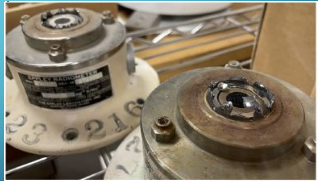
Photograph of Eppley PIR pyrometers with broken domes from improper packing when shipping. Photo credit L. Riihimaki
