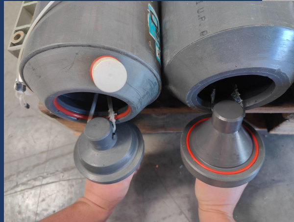
General niskin (left) vs Bullister-style (right)
