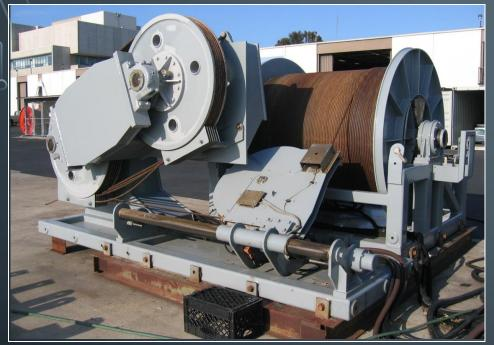
Dynacon Traction Winch Up to 25,000 lbs pull. Holds 10,000 m of .681 cable.
