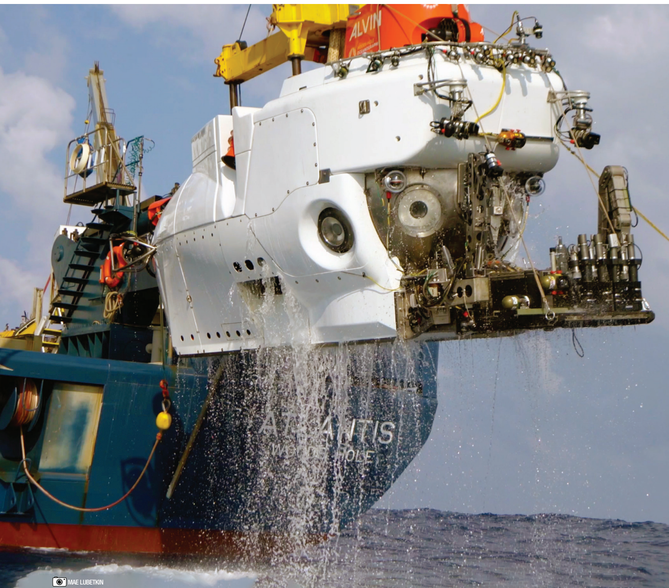
Figure 25: Alvin being recovered by RV Atlantis , from a dive in March 2024 during expedition AT50-21. Four MISO GoPro camera systems are mounted on the submersible, in addition to two DeepSea 4K Optim cameras on port and starboard pan and tilt systems (see also Figure 13).
