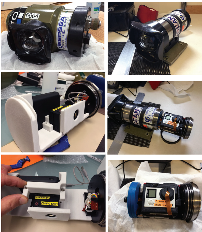
Figure 3: MISO GoPro™ camera systems, 1st and 2nd generation cameras that use GoPro HERO4™ imaging modules. Left panel shows the 1st generation system in the DeepSea Digi SeaCam housing and right panel shows the 2nd generation cameras in the DeepSea Super SeaCam housing, both rated to 6,000 m operating depths.
