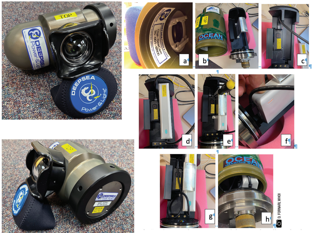
Figure 4: 3rd generation MISO GoPro™ camera system which uses a GoPro™ HERO11 camera module in a new (2024-manufacture) DeepSea Digi SeaCam housing (6,000 m rated). Left panel shows two views of the new housings. Right composite image shows the internal chassis that holds the HERO11 camera and aligns it to the housing optics, internal USB battery and cabling and associated components. Installation of the HERO11 and USB battery and set-up of the camera pre-dive takes ~15 minutes. When the camera is deployed on a vehicle in hot, tropical weather, care must be taken to cool down the housing so that the camera module does not overheat – this is especially true for 5.3K or 4K video recording.
