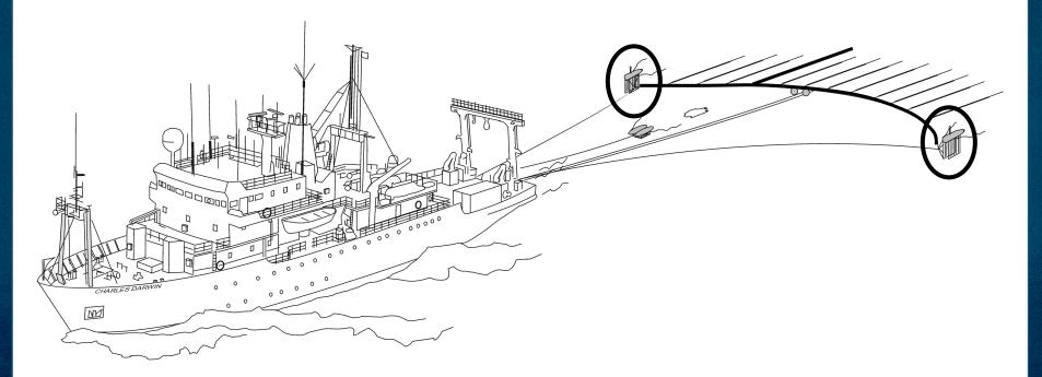
A seismic cable towed perpendicular to the vessel's steaming direction Many single-channel seismic streamers attached to a wire held in place by two doors
