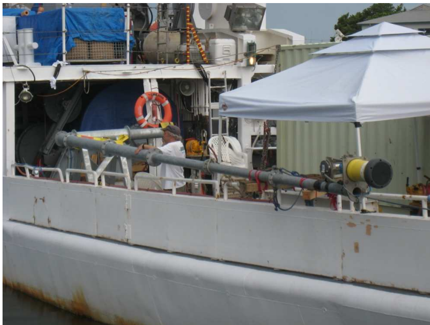
Figure 37 - USBL pole retracted and secured in the stowed position. To deploy, a crane is used to hold the near end, the assembly slides outboard relative to the base, and is rotated clockwise into the water where it is locked in the down position.
