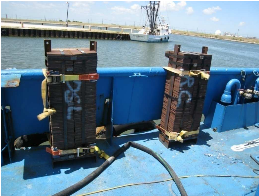
Figure 34 - Weight stacks secured to the side rail of a ship
