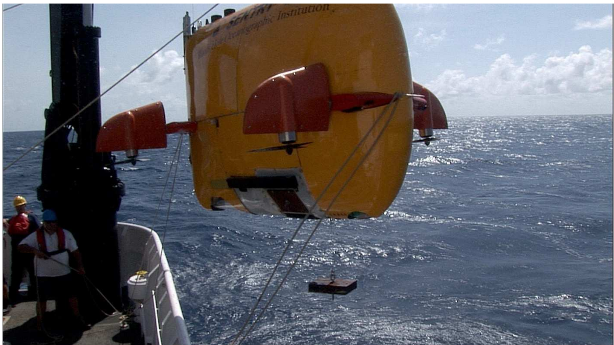
Figure 43 - As Sentry moves over the rail, the forward tagline is slacked and slipped.
