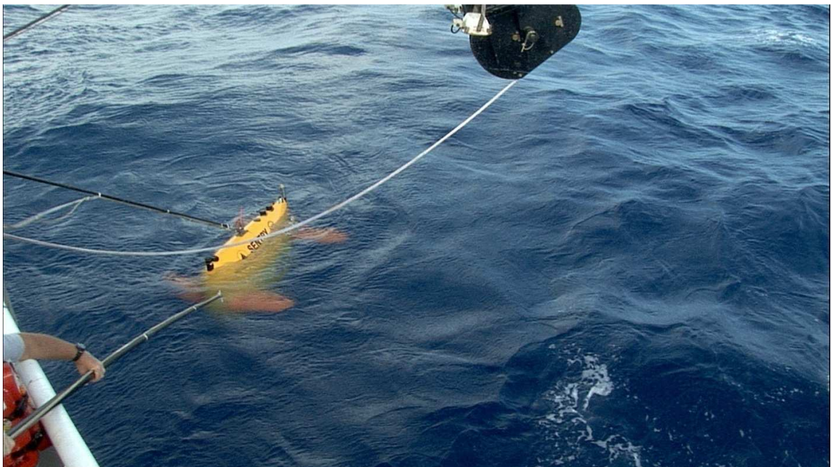
Figure 45 - As the vehicle drives towards the stationary vessel, the lift line for the crane is attached using a carbon fiber pole. The vehicle immediately drives full reverse and the pole is potentially used to fend the vehicle while the lift line is tensioned.
