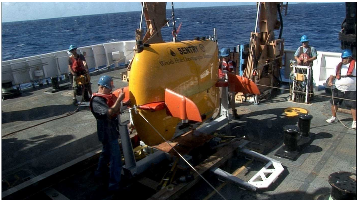
Figure 47 - The vehicle is slewed back into the cradle and the fore and aft catches are secured first. The side is reattached and the poles reinserted before the vehicle is set into the cradle.
