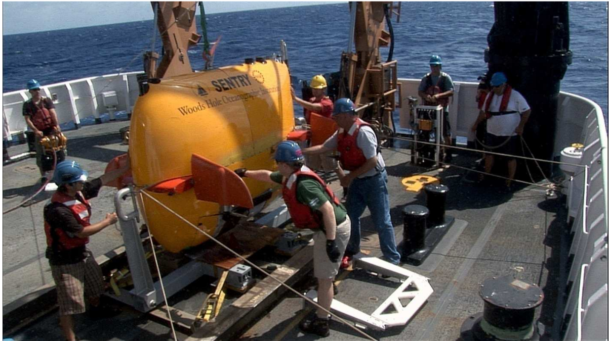
Figure 40 - The outboard side of the cradle is removed and the pipes through the center of the vehicle are removed.
