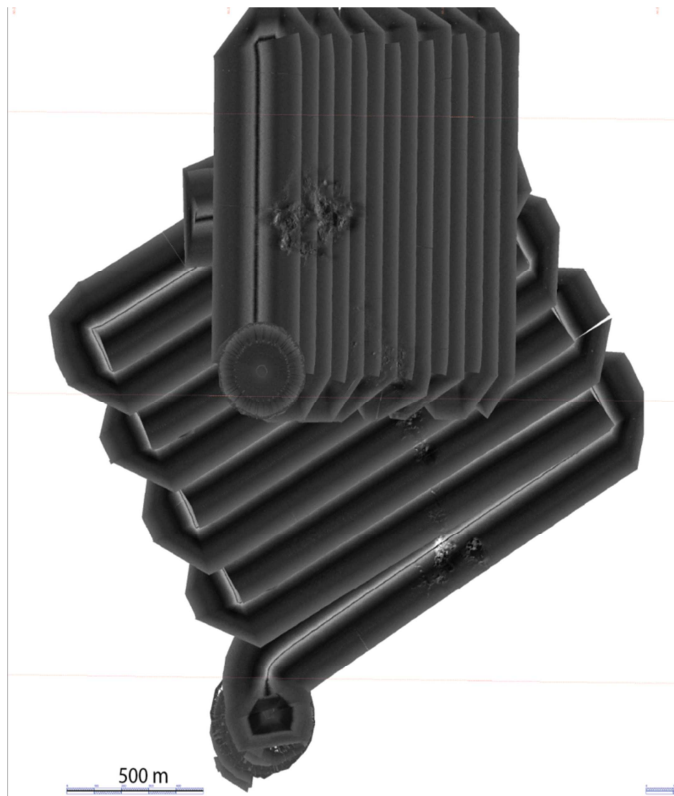
Figure 24 - Example of a rough sidescan mosaic. These are typically easy to make but do not deal elegantly with overlap, nadir, etc. Data from Cindy Van Dover and Laura Brothers
