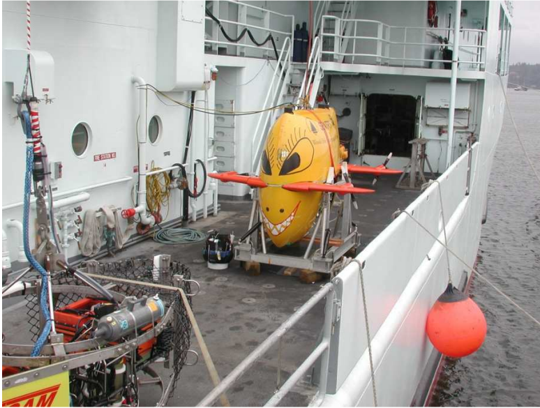
Figure 33 - Typical location of the Sentry Cradle . Note the cables running from the wall to the vehicle, the ample work room around the vehicle, and the proximity to the side of the ship relatively close to the water.
