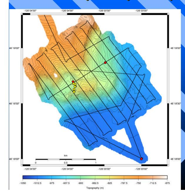
50 m altitude 150 m spacing Hydrate outcrops (yellow dots) perched on plateau 150 m above the canyon floor Red dots show planned Neptune-Canada cable nodes. 5 m contours Ø
