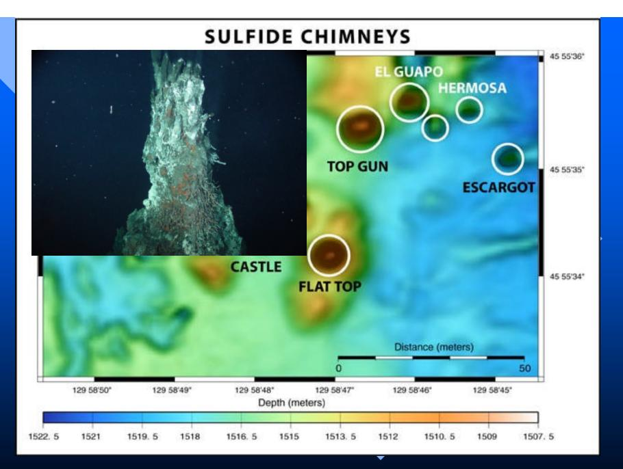
AUV bathymetry showing 7 newly discovered active sulfide chimneys on the <sup>18</sup> east side of caldera. This map guided ROV ROPOS operations.
