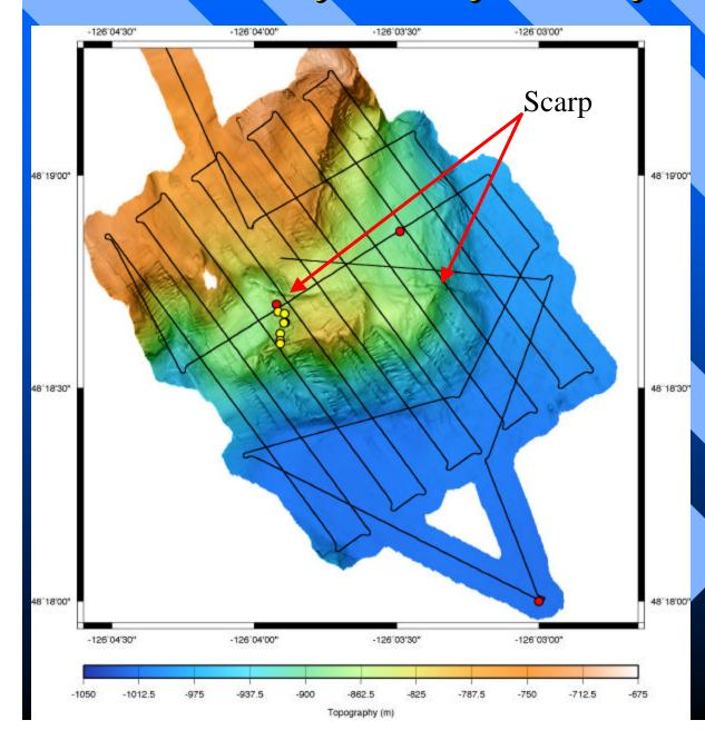
Slope shading w/1 m lateral resolution reveals a 5-15 m high scarp cutting across the plateau ∠ Newly discovered feature is apparently an active reverse fault Possibly explains the location of the hydrates
