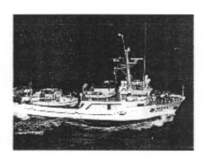
RUDE (\$590) is a 90-foot survey vessel outfitted for hydrographic surveys. The vessel specializes in wreck and obstruction investigations in support of the nation's nautical charting program. The RUDE is outfitted with a shallow water multi-beam sonar system enabling it to survey large bottom areas in a single pass. This vessel normally operates along the Atlantic and Gulf coasts. Its home port is Norfolk, Va.
